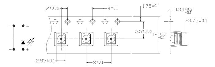
**Note:** Tolerances Unless Dimension  $\pm 0.1$ mm Unit = mm
